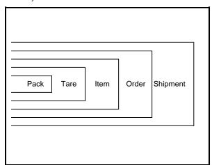
Each box represents one hierarchical level and associated data segments detailed in this explanation. Required hierarchical levels are represented.
